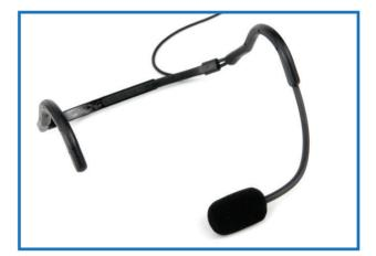
The construction of this headband microphone offers a high degree of protection against the ingress of sweat. Precise placement is obtained with the 4mm diameter flexible gooseneck, and the condenser capsule is highly efficient at noise cancellation - helping prevent feedback or interference from crowd noise etc. This slim line Aerobic Headset is available in a choice of the following colours: Black, Blue and Yellow.
